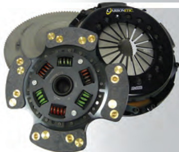
The small-diameter Carbonetic clutch reduces clutch mass for improved engine response and quicker transients while still offering the torque-holding capacity of a large diameter unit.
